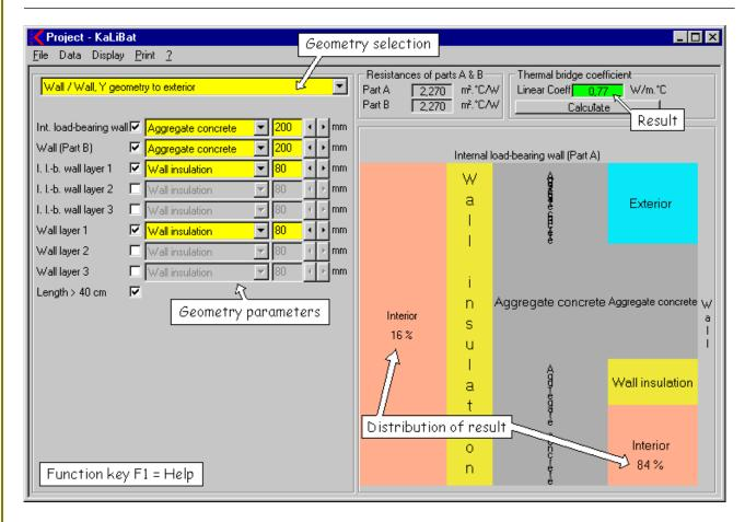
KaLiBat has a graphic interface allowing an immediate visualization of the geometry, with its data. Its use is similar to that of a calculator.
